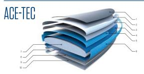
1- Deck Pad. / 2&10- Thermoformed plastic skin (ASA). / 3- 50g/m² Fiberglass wrap. 4&8- 200g/m<sup>2</sup> Woven Fiberglass. / 5- 200g/m<sup>2</sup> Woven Fiberglass Reinforcement Patch in standing area. / 6 -200g/m2 Woven Fiberglass Rail Reinforcement. 7- Molded, Watertight EPS Foam Core. / 9- 50g/m2 Fiberglass wrap.
